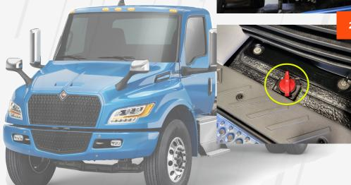
High voltage in Zone 1 can be isolated when the High Voltage Disconnect switch is in the "OFF" position.
