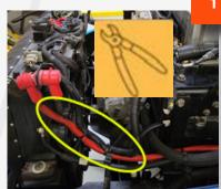
Isolating the 12V system can be accomplished via the Low Voltage Disconnect switch **OR** by cutting the main red battery cable located under the hood.
