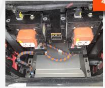
High voltage in **Zone 2** is electrically isolated when **Level 2 MSDs are** disconnected.
