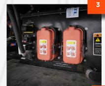
High voltage in **Zone 1** is electrically isolated when **Level 1 Manual Service Disconnects (MSDs)** are disconnected.
